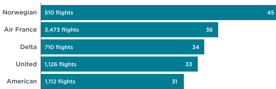
Figure 7. Fuel efficiency (pax-km/L) for airlines serving New York-Paris routes.
